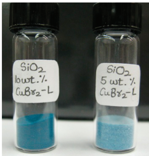
Figure 2. Vials containing catalyst complex ( \text{CuBr}_2/\text{PMDETA} ) physically adsorbed on silica gel \text{Cu}^{\text{II}}/\text{silica} = 10 and 5 wt %.
